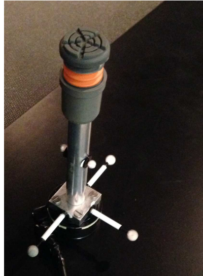
Figure 3 - The device developed to test the force platform.
