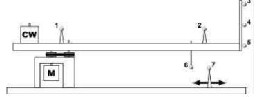
**Figure 1.** The device used in testing. Markers 3 – 5 are mounted on a plate at the end of the arm, preventing these markers from being seen by all cameras at once. Marker 6 passes near Marker 7 once per revolution, making resolution of these markers challenging.
