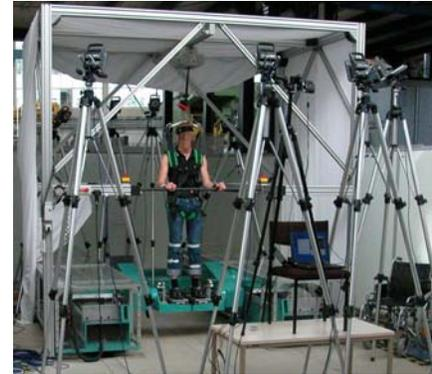
Figure 1: Rehabilitation robot *HapticWalker* with optical system
