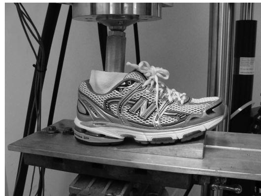
All shoes were initially tested monotonically to determine time zero stiffness. Each brand of shoe was tested dynamically up to 600 miles and monotonically at 5, 10 15, 25, 50, and
