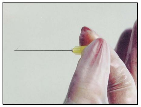
Figure 12 - Fine Wire Electrode
