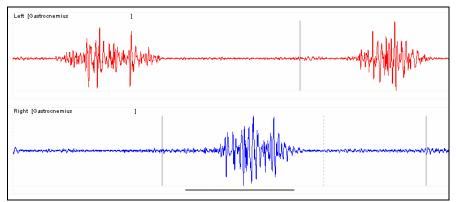
Figure 7 - EMG recorded at the correct level is large enough to be analyzed but does not clip.
