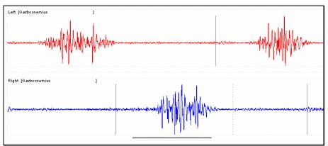
Figure 5 - An EMG signal showing clean muscle activation (recorded with an MA-300).
