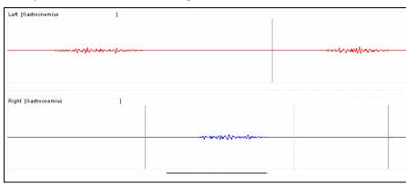
Figure 8 - EMG recorded at too low a level is difficult to observe or analyze.
