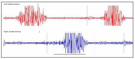
Figure 9 - EMG recorded at too high a level is distorted and provides limited information.
